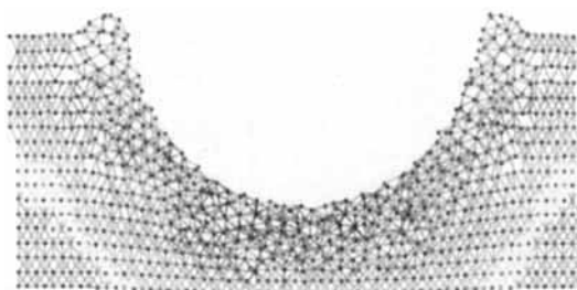
FIGURE 5 Illustration of the distribution of average shear stresses at maximum indentation depth. (See Color Plate I).
